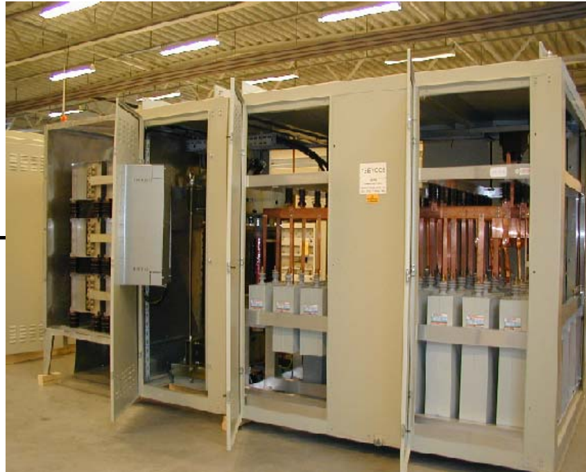
Direct Electric Heating Topsides
