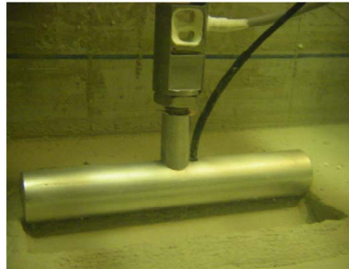
Pipe model during testing
